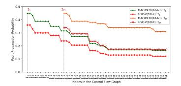
Figure 10: The fault propagation probability of instructions  $I_1$ ,  $I_{15}$  for the processors TI MSP-430(16-bit) and RISC-V(32-bit) for the toy cipher implementation given in Figure 3.
