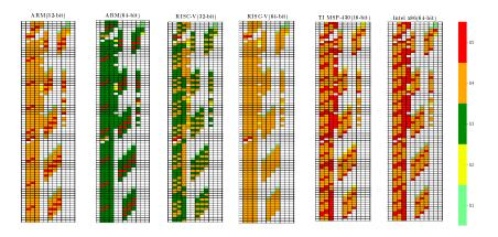
Figure 11: SuccessScore of vulnerable instruction from an AES(LookUp Table) based implementation on six different processors. Each cell represents an instruction and the color code represents the SuccessScore.
