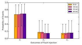
$\left( d\right)$  Probability of events when a transient fault is injected in a register or data memory operand
