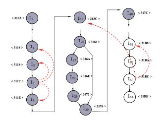
**Figure 6:** Control Flow Graph (CFG) with addresses ( $\langle \cdot \rangle$ ) for the intermediate representation of the pseudo-code given in Figure 2. The addresses correspond to an implementation on TI's MSP-430, while the shaded nodes are vulnerable. A fault in the program counter can skip instructions or repeat the execution of instructions as shown by the dashed lines.
