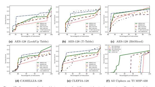
Figure 12: Percentage of vulnerable instructions for different cipher implementations. To understand these graphs, consider for example in Figure (d), when x = 85%, y = 0.38 on TI MSP-430(16-bit). This means that 85% of CAMELLIA-128 instructions have SuccesScore  $\leq 0.38$ .
