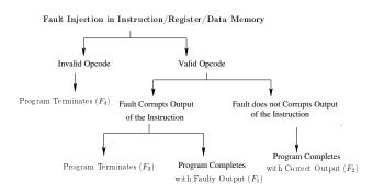
**Figure 4:** Manifestation of a fault injected in instruction or data may either alter or leave unaltered the instruction output. It may also result in a program termination.
