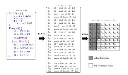
**Figure 3:** Vulnerable Instruction Identification. The Intermediate Representation obtained from the LLVM compiler for the pseudo code is used by FEDS to identify vulnerable instructions.
