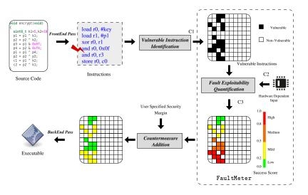
**Figure 1:** The FaultMeter framework, to quantify the vulnerability of block cipher implementations. It has two main modules. The Vulnerable Instruction Identification Module detects vulnerable instructions, while the Fault Exploitability Quantification module quantifies the exploitability. The figure also shows an application of FaultMeter to automatically insert countermeasures into the implementation. The countermeasures are tuned to meet the user's security requirement.
