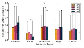
(b) Probability of producing an incorrect output for different fault models in RISC-V (32-bit)
