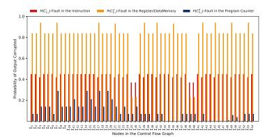
**Figure 7:** The probability of a fault corrupting the output of instructions given in Figure 3 on an TI MSP-430 processor. Faults can be induced either in the instruction, memory, or in the program counter.
