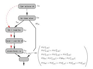
Figure 9: Fault propagation across the control flow instruction can corrupts the store instruction  $I_{29}$  either through data-dependent sequence (marked in red) or by a fault in branch  $I_{26}$ .
