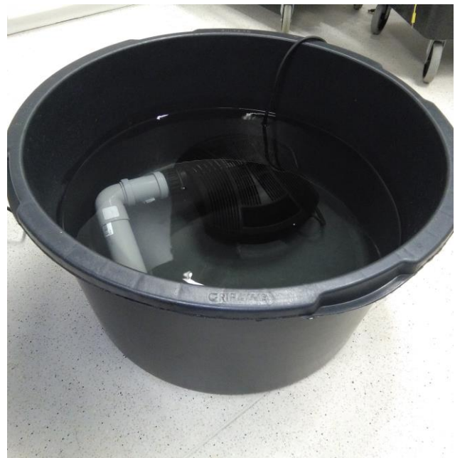
Fig. 2. Picture of the water pump placed inside a circular container filled with water
