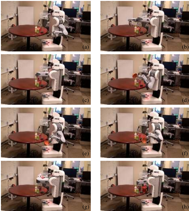
Fig. 7: The PR2 robot picks up a bowl and moves it to the side before placing it back on a table while avoiding all other objects in the environment. FCL is used as the collision library and integrated with motion planning and kinematics modules used in this task.
