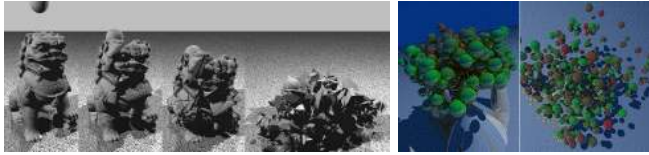
Fig. 5: Non-rigid benchmarks used for performing CCD and self-collision queries in FCL. In the left benchmark, a stone falls on top of a Chinese lion model and the lion gradually breaks into a high number of colliding pieces. The benchmark has 1.6M triangles with 45 frames. The right benchmark consists of multiple moving objects. Each object undergoes deformable motion, and the objects collide with each other and the ground. It contains 146K triangles with 94 frames.
