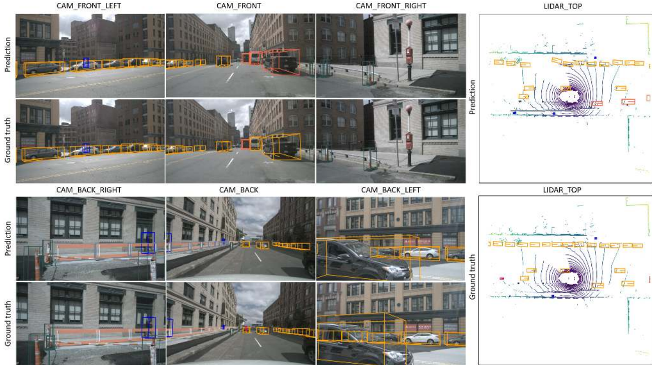
Figure 5: Qualitative analysis of detection results. 3D bounding boxes predictions are projected onto images from six different views and bird-view, respectively. Boxes from different categories are marked with different colors. We can see that the results are reasonable except for some detection with false class predictions from the left part. Moreover, a few small objects are detected by our model while not annotated as ground truth, like barriers in the back/back right camera. However, apart from the inherent occlusion problem in this setting, depth and orientation estimations of some objects are still inaccurate, which can be observed in the visualization from bird-view.
