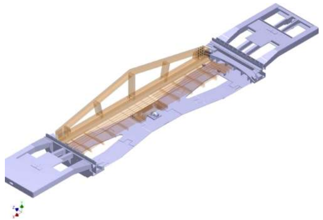
Fig. 2. Simplified 3D geometrical model – a view with a cross-section of a rotatable platform
