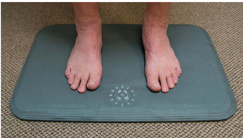
Figure 1 —The study device was an in-home, wireless, thermometric mat designed for remote temperature monitoring of patients at risk for inflammatory foot diseases.
