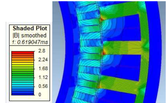
Fig. 3. FE model of the best performing machine after SR and tooth width studies.
