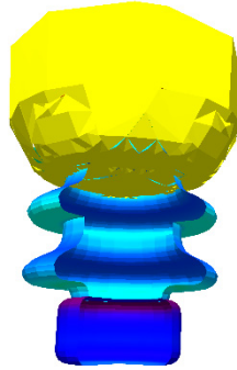
Figure 9: Isosurface of the electric potential.
