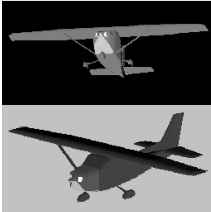
Figure 5: SPIRITS MWIR Image of Cessna 172 against Lowtran MLS atmospheric background. The upward view shows net positive contrast, the downward view net negative contrast.
