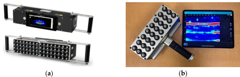
Figure 8. PAU systems used: (a) A1040 MIRA 3D (two devices were attached side by side to increase the number of channels to 16 rows of 4 transducers each) [115], (b) Pundit live array pro.
