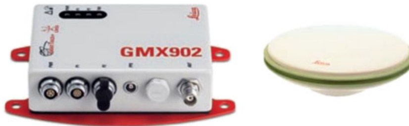
Figure 3. Leica GMX902 dual-frequency GPS receiver (left) and AX1202 antenna (right): 0.2 mm RMS accuracy, 2.4 W power consumption, and up to 20 Hz sampling rate [30].
