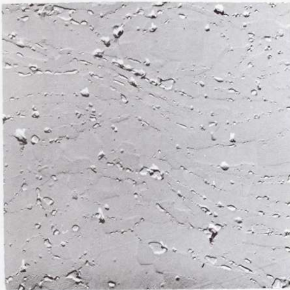
(c) Ball-milled in HI; run 5, tables II and III; interparticle spacing, 2.1 micrometers.
