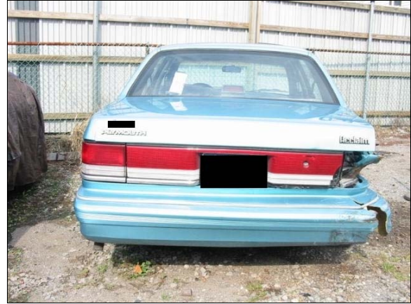
Figure 6. NASS/CDS Case 2004-08-162 the rear damage to Vehicle 2
