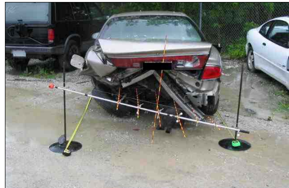
Figure 3. NASS/CDS Case 2004-12-081 the rear damage to Vehicle 2
