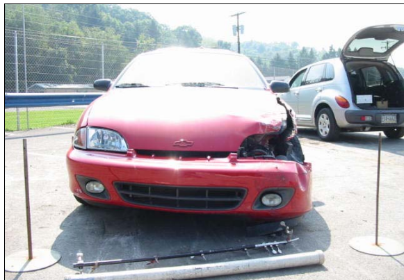
Figure 5. NASS/CDS Case 2004-08-162 frontal damage to Vehicle 1
