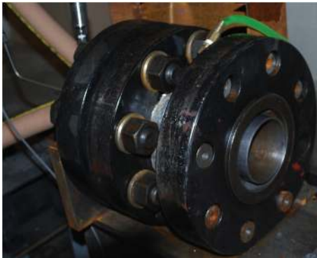
FIGURE 4: Photograph of the battleship motor casing for 3'' diameter propellant grains.
