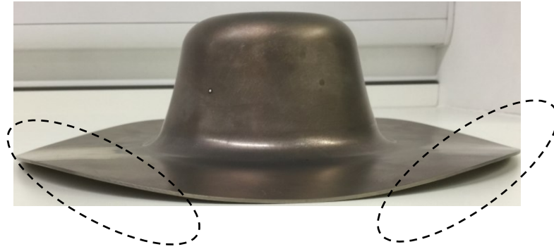
Fig. 10. Hydroforming stage 2 Formed part showing the flange distortion.
