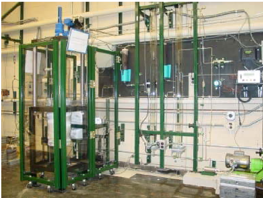
Figure 29. Photograph of the SCW loop.
