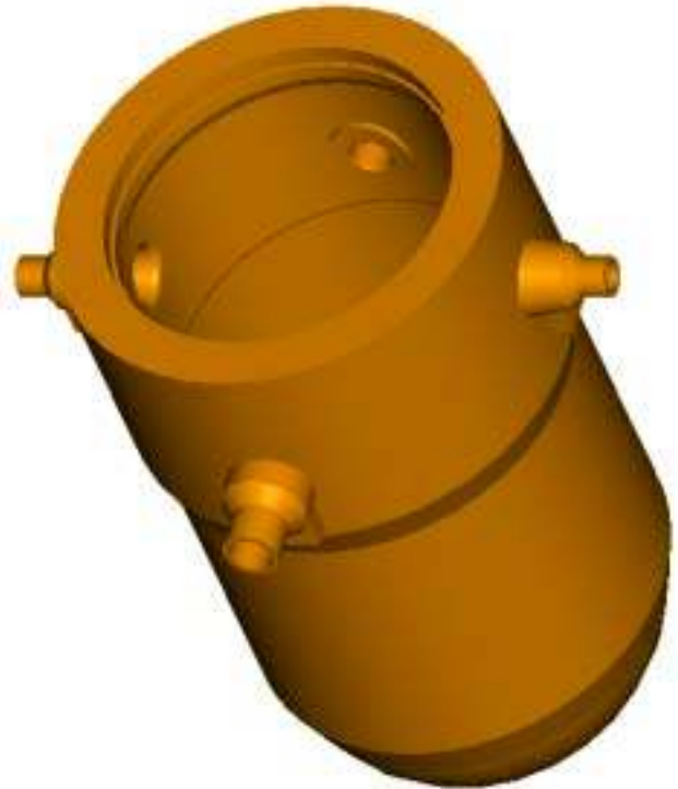
Figure 2. Three-dimensional cad-com representation of the current SCWR pressure vessel design.
