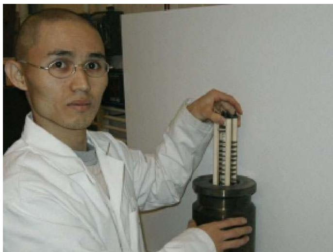
Figure 7. The rack of samples is inserted into the Inconel 625 exposure vessel prior to an experiment.
