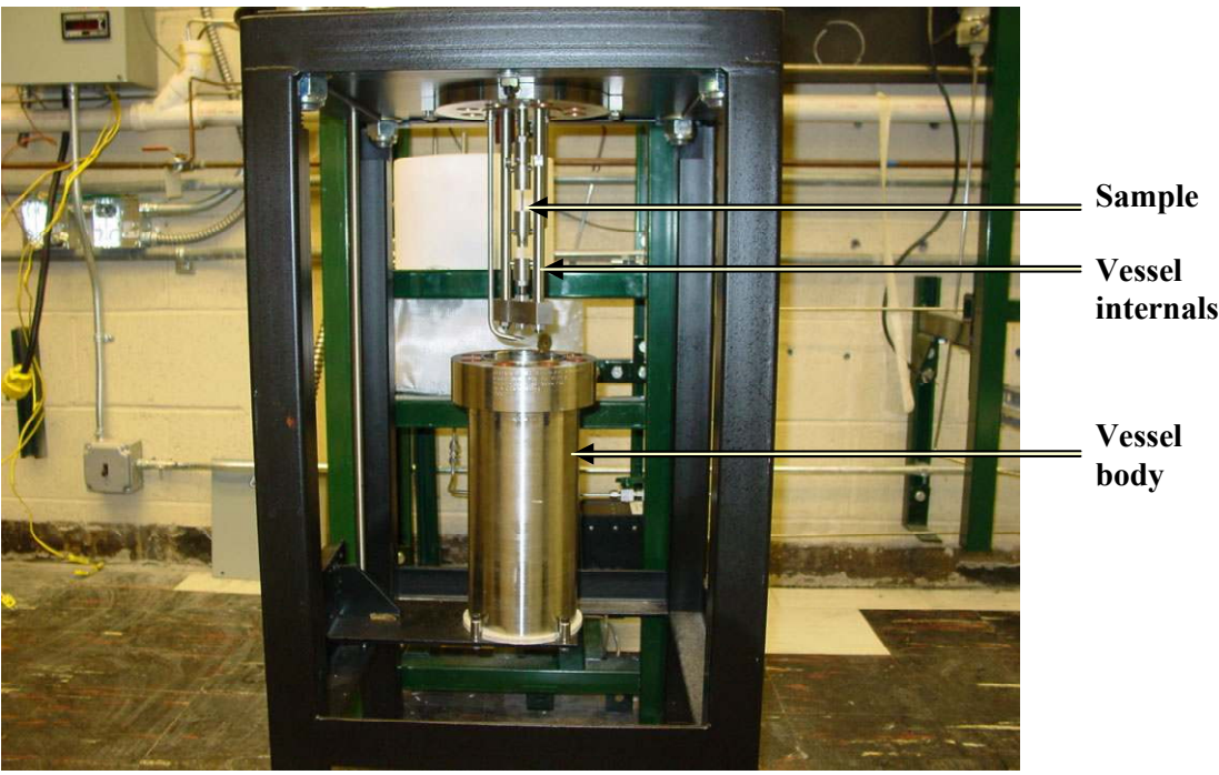
Figure 11. Supercritical water system: autoclave vessel and internals.
