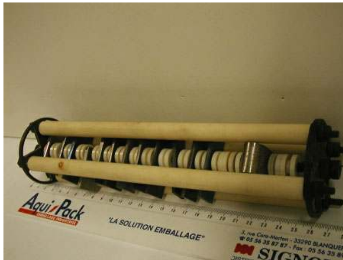
Figure 6. The sample rack that will be used during the MIT exposure studies. The samples are electrically isolated from each other and the rack by means of alumina spacers.
