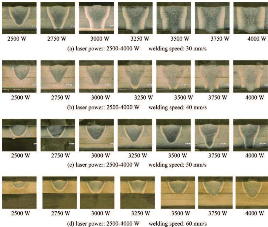
Fig. 14 Cross-sectional view of the penetration depths with different laser welding parameters (magnification 4 \times )
