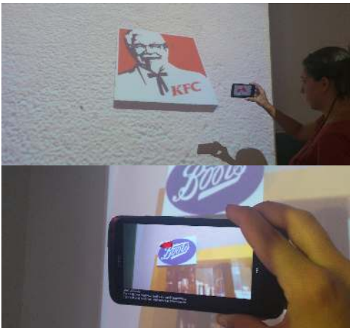
Figure 16. Scanning indoor features in a virtual environment. The navigation instructions and directional arrow are visible in the lower image.
