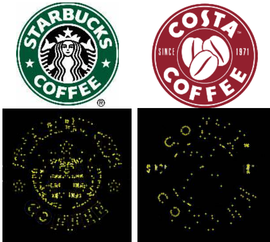
Figure 2. Two optically “similar” logos from actual businesses within a mall. After feature detection, it can be seen that it is easy for a system to distinguish between the two
