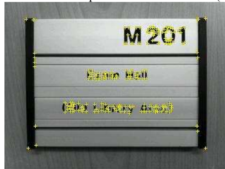
Figure 1. Visible features of a door sign via Qualcomm Vuforia SDK
