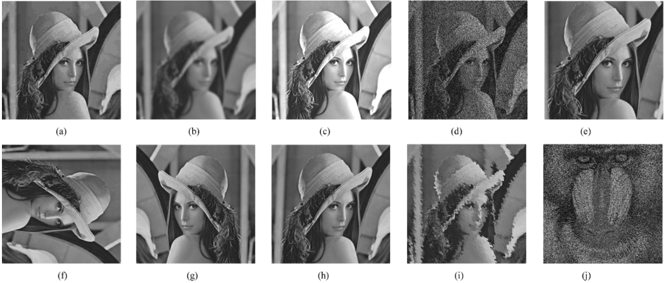
Fig. 4. Similarity values obtained from the PSNR, VIF, and our FSRISA between the Lena image and its manipulated images. (a) JPEG compression (PSNR = 30.87 dB, VIF = 0.31, FSRISA = 0.73). (b) Blurring (PSNR = 25.17 dB, VIF = 0.13, FSRISA = 0.60). (c) Brightness and contrast adjusting (PSNR = 15.41 dB, VIF = 1.06, FSRISA = 0.67). (d) Noising (PSNR = 12.05 dB, VIF = 0.08, FSRISA = 0.50). (e) Scaling and cropping (PSNR = 13.71 dB, VIF = 0.02, FSRISA = 0.67). (f) Rotation (PSNR = 11.66 dB, VIF = 0.01, FSRISA = 0.77). (g) Flipping (PSNR = 11.83 dB, VIF = 0.02, FSRISA = 0.53). (h) Shearing (PSNR = 18.00 dB, VIF = 0.07, FSRISA = 0.57). (i) Rippling (PSNR = 22.18 dB, VIF = 0.07, FSRISA = 0.49). (j) Irrelevant image (PSNR = 9.69 dB, VIF = 0.02, FSRISA = 0.04).
