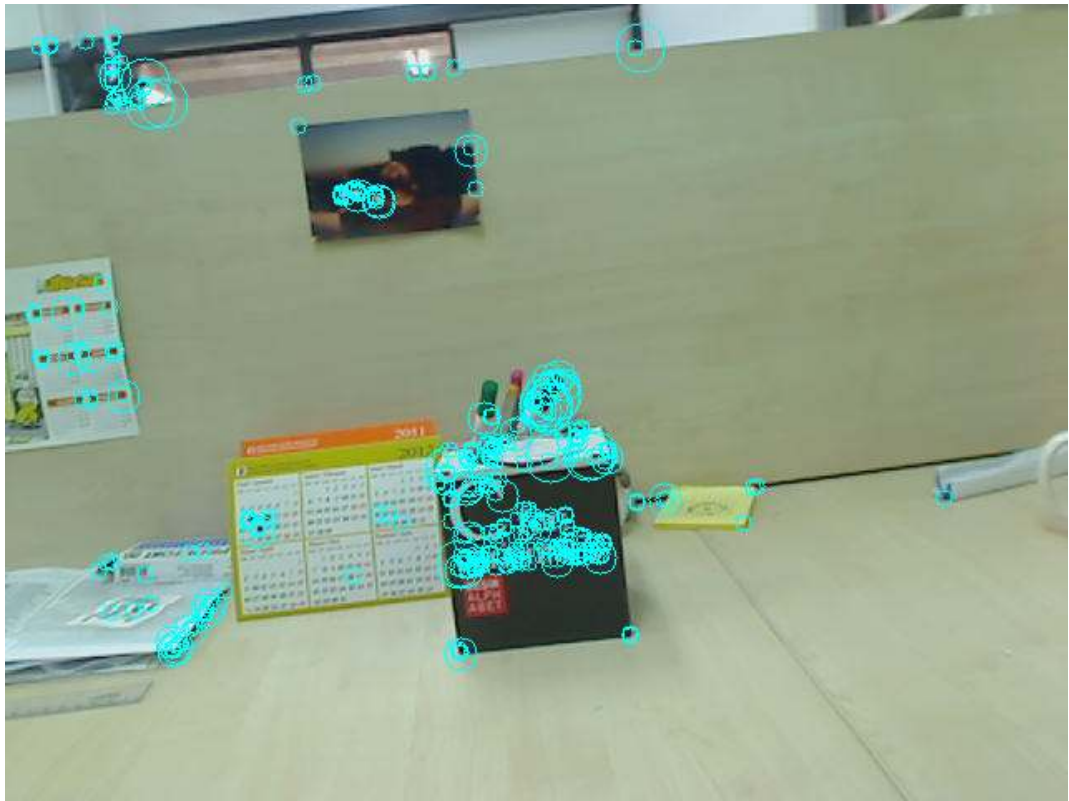
Figure 35 A sample capture from the webcam. The diameter of the circles represents the scale of the detected points.
