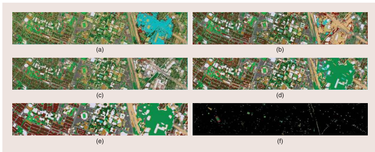
FIGURE 11. The classification maps obtained on the extracted features from Houston University 2013 data set: (a) HSI, (b) OTVCA, (c) JPlay, (d) CNN, (e) PCNN, and (f) ground reference. From each category, the method with the highest OA is shown for the demonstration, and (a) is the one obtained from the spectral bands.
