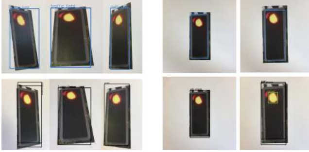
Fig. 5. (Left) Adversarial examples in physical domain remain adversarial at multiple angles. Top images classified correctly as traffic lights, bottom images classified incorrectly as either ovens, TV screens, or microwaves. (Right) Adversarial examples in the physical domain remain adversarial at multiple scales. Top images correctly classified as traffic lights, bottom images classified incorrectly as ovens or microwaves (with the center light being misclassified as a pizza in the bottom right instance).
