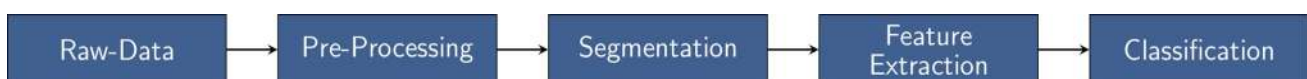
Fig. 1 The Activity Recognition Chain (ARC) in conventional ML approaches. Adapted from Bulling et al. (2014)
