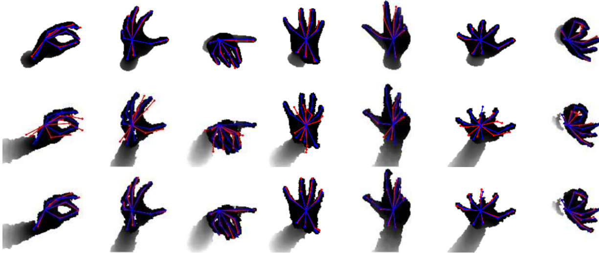
Figure 6: Qualitative results on the NYU dataset [45]. Top row: Predicted poses on synthetic test depth maps, and Middle row: predicted poses on real test depth maps, when training on synthetic depth maps only. Training only on synthetic depth maps does not generalize well to real depth maps. Bottom row: Predicted poses when using our method. We plot the 2D projection of the 3D pose prediction. Blue denotes ground truth annotations, red are our predictions.
