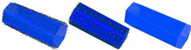
Fig. 12 Reconstruction and simplification of a cylinder. Left: 10K noisy sample points and reconstruction with 12 vertices (facet density shown). Middle: transport plan between point samples and bin centroids. Right: simplicial complex and facet density.
