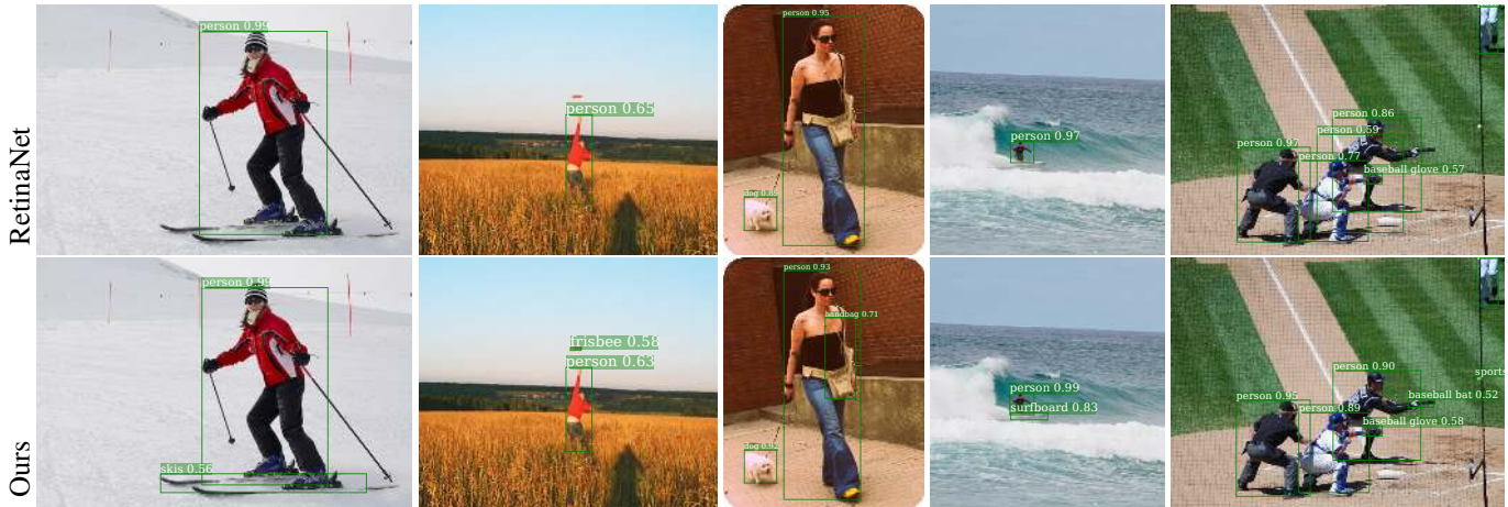
Figure 7: More qualitative comparison examples between anchor-based RetinaNet (top, Table 1 1st entry) and our detector with additional FSAF module (bottom, Table 1 5th entry). Both are using ResNet-50 as backbone. Our FSAF module helps finding more challenging objects, such as thin objects (skis, frisbee, handbag, surfboard) and small objects (baseball).
