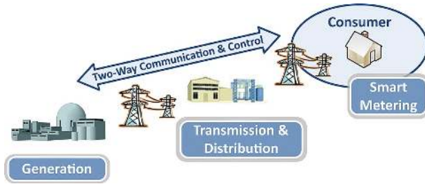
Fig.1: Two Way Communication in Smart Grid [41].
