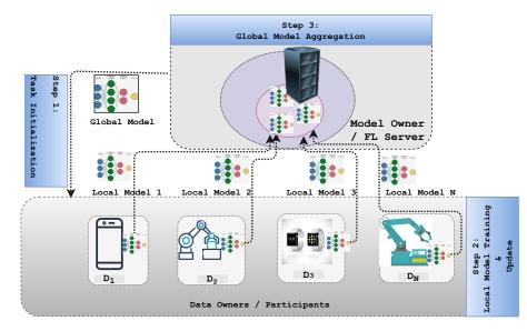
**Figure 3.** An FL general process with the server and N participants synchronizing with a server and updating it with an updated global model in a single communication round.
