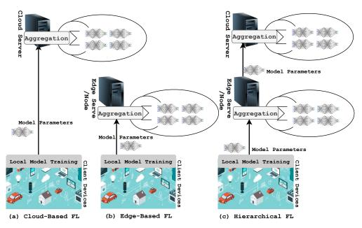
**Figure 1.** Three federated learning structures: (**a**). Cloud-enabled, (**b**) edge-enabled, and (**c**) hierarchical (client-edge-cloud-enabled).
