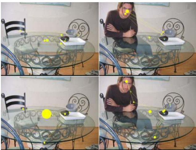
Fig. 1 Different scanpaths on a pair of images eye tracked from different human observers. Left , free viewing of a natural scene; right , natural scene embedding a face. The area of yellow disks marking fixations between saccades is proportional to fixation time (images from the Fixations in FAcEs dataset)
