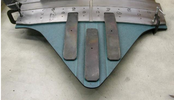
Figure 3: Chevron during final assembly.
