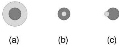
FIG. 32. Light beams and pupil sizes. Light beam is shaded light; pupil is shaded dark. (a) The ordinary case: the beam is larger than the pupil. (b) Breaking the feedback loop: the beam is smaller than the pupil. (c) Inducing pupil oscillations: a small beam falls on the edge of the pupil.
