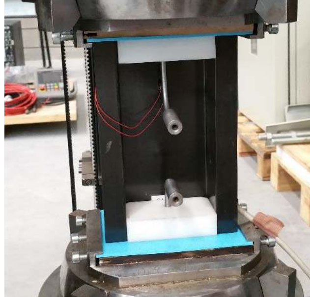
Fig.2. Boundary conditions: a) C-shape section sample, b) \Omega -shape section sample.
