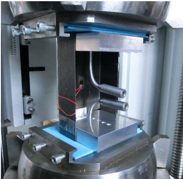
Fig.2. Boundary conditions: a) C-shape section sample, b) \Omega -shape section sample.
