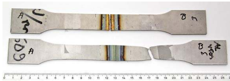
Figure 15 Samples from the tensile tests showing an autogenous TIG-welded specimen in grade 1.4016 which demonstrated a brittle weld metal fracture (top) and also a ductile base metal fracture in an autogenous TIG-welded specimen made from Grade 1.4509 (bottom).
