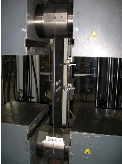
Figure 16 Tensile test sample of a bolted connection test on Grade 1.4509 ferritic stainless steel with a thickness of 1 mm
