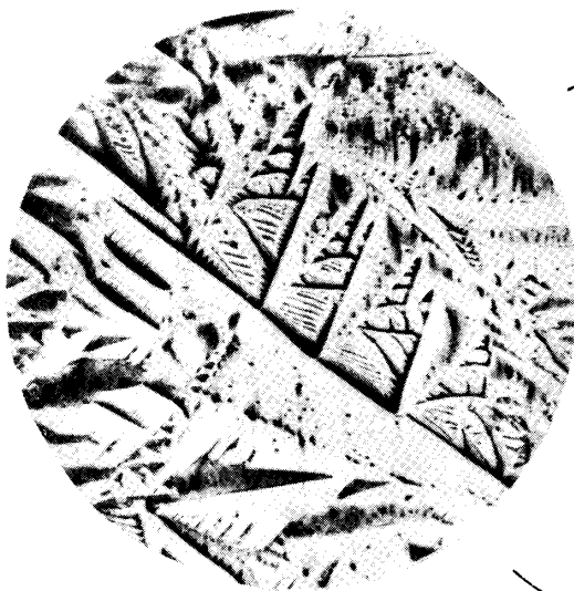
Photo. 9. Domain patterns on the crystal surface closer to the (110) plane than in Photo. 8.
