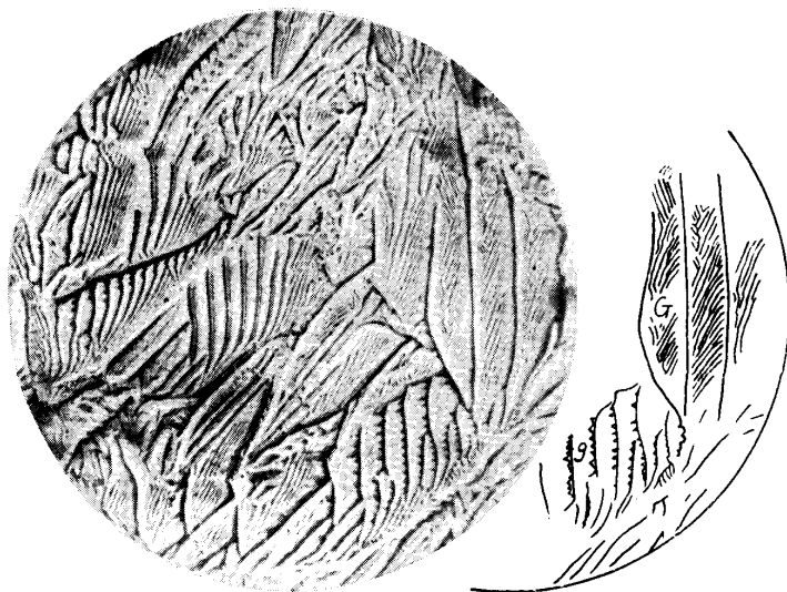
Photo. 12. Domain pattern on the crystal surface slightly inclined from the (100) plane towards the (211) plane.
