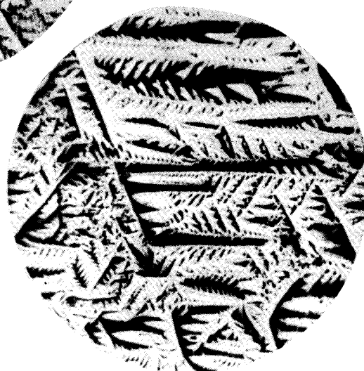
Photo. 19. Domain pattern on the crystal surface inclined slightly from the (111) plane towards the (211) plane.
