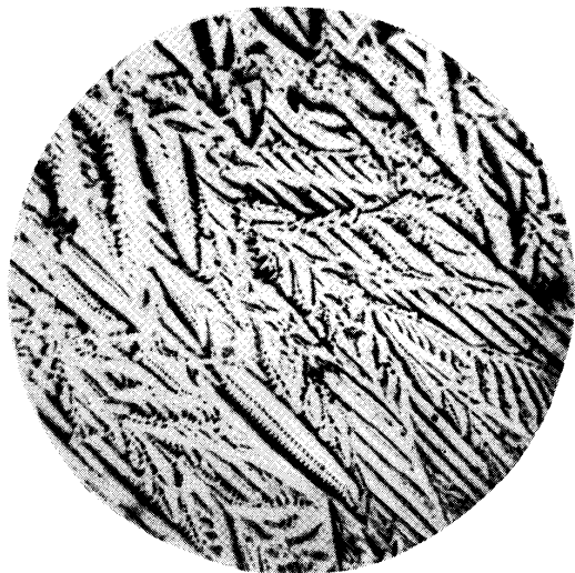
Photo. 15. More complicated second-kind tree pattern observed on the crystal surface inclined further than in Photo. 14.
