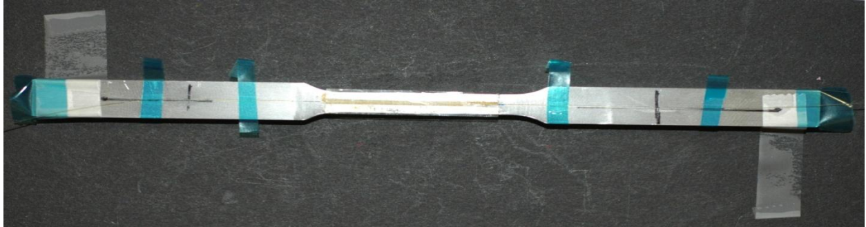
Figure 5, FBG array bonded Al alloy sample
