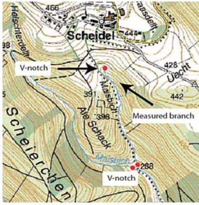
Figure 1. Topographic map of the Maisbich, indicating the positions of the upper and lower v-notches, which are 600 m apart.
