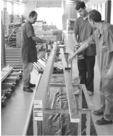
Application of glue on sheets.
