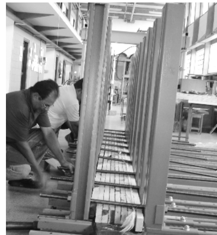
Pressing of beam with reinforcement.
