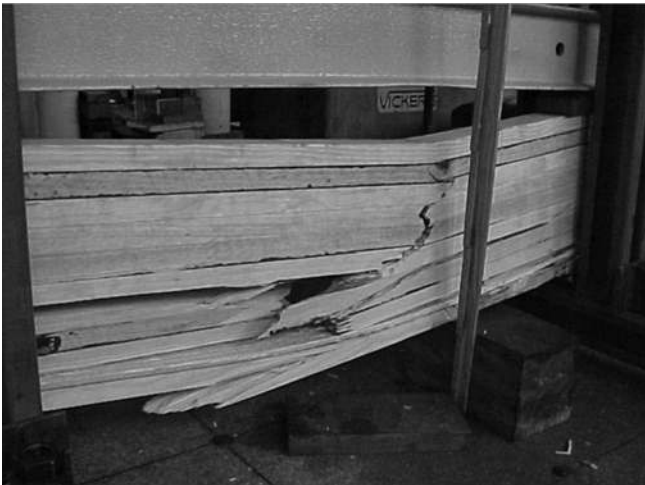
Figure 8. Rupture modes of the experimentally evaluated glulam beams.
