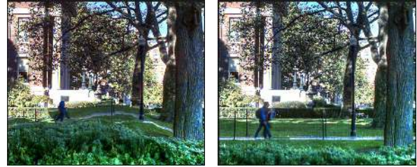
HDR Image (exponential) HDR Image (Fibonacci) Figure 10. Evaluating the effect of non-linear camera response. A non-linear response was emulated by applying a \gamma -curve ( \gamma = 2.2 ) on the input LDR frames. Because of differences between exposures of consecutive frames, there are strong distortions for exponential (bushes, walking path and people at the bottom) scheme. In contrast, the proposed approach is robust to non-linear response.
