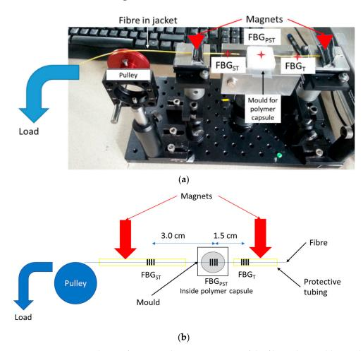
**Figure 3.** Experimental setup for testing the strain response of the fibre. The mould provides an anchor point to isolate  $FBG_T$  from the effects of strain, the magnets hold the yellow protective tubing in place and the rest of the fibre can slide within the yellow jacket. (a) Labelled photograph; (b) labelled schematic.
