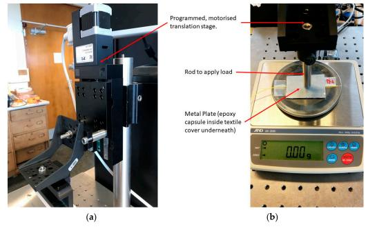
**Figure 2.** Customised calibration setup. (**a**) The motorised translation stage is programmed to lower the rod onto the weighing scale. The pressure sensor in its textile housing is attached to the plate of the weighing scale to keep it in place during the calibration. (**b**) The load is transferred from the translation stage to the pressure sensor via a metal rod and an aluminium metal plate. The probe is lined up over the central FBG of the sensor before starting the loading process.
