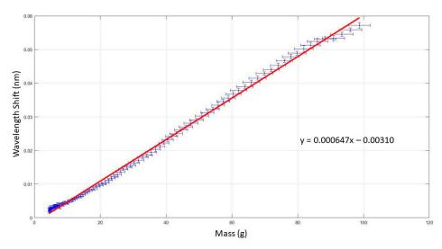
**Figure 7.** Typical calibration results of the FOPS: wavelength shift against load weight using experimental set up illustrated in Figure 2.
