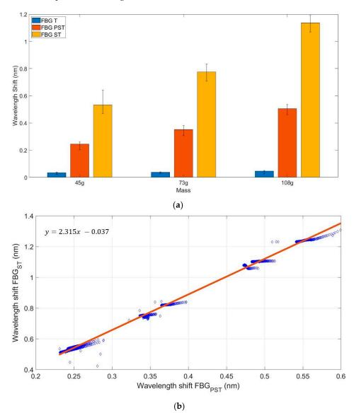
**Figure 8.** (a) Typical response of the 3 FBGs to the load applied for strain compensation measurements (using experimental set up in Figure 3), showing the mean wavelength shift for each applied mass.
