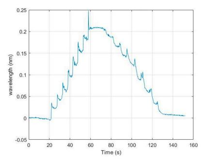
**Figure 10.** Typical results: wavelength shift against time underneath a compression bandage wrapped multiple times (in this case 8 layers) on a single location on the phantom leg. The displayed wavelength values are strain and temperature compensated.
