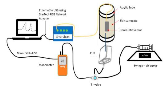
**Figure 4.** Experimental setup for measurements using a blood pressure cuff. A controlled volume of air is added via syringe pump to the cuff, which is wrapped around the materials on the acrylic tube. The pressure of the cuff is recorded by the manometer and is compared to the wavelength shift recorded by the interrogator.
