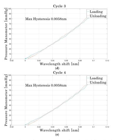
**Figure 9.** (a) Typical results: comparison of wavelength shift produced by the sensor to the pressure from a manometer, taken on a rigid cylindrical tube and controlled by a blood pressure cuff (using the experimental set up in Figure 4). (b–e) Pressure against wavelength shift for four loading and unloading cycles.
