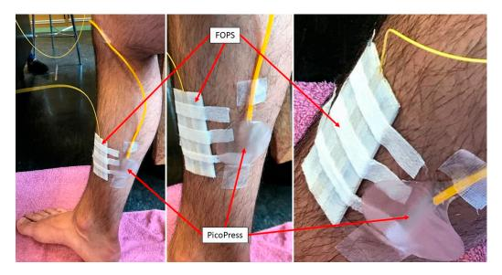
**Figure 6.** Photos of the optical fibre sensor and the PicoPress at approximately the B1 position on a human subject.
