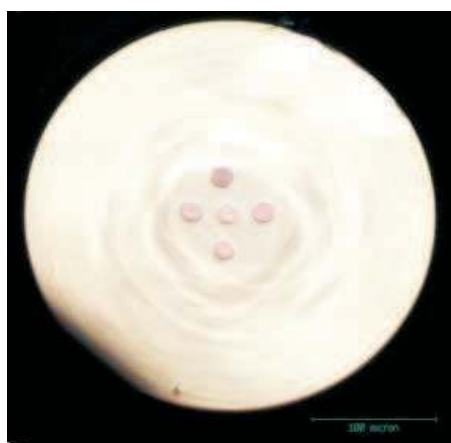
Fig. 15. Cross section (left) and luminescence spectra (right) of the fabricated multicore fibre
