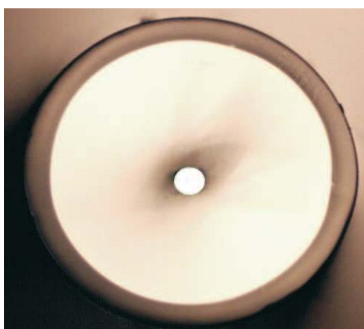
Fig. 16. Cross-section of tellurite optical fibre moped with Yb^{3+}/Tm^{3+} (1:0.1 mol%), core/cladding diameter 40\mu m/450\mu m
