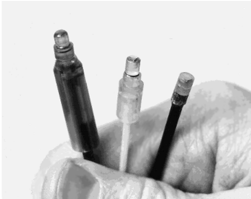
Fig 39. Three versions of multimode sensors with folded design
