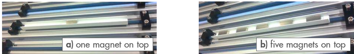
Figure 9.5: Magnet assemblies incorporating (a) one magnet and (b) five magnets as used in the laboratory reliability tests. The overall length of the five-magnet assembly is 0.4 m. Also note the fibre-optic cable underneath and the mounting clips used to immobilize the cable onto the substructure.
