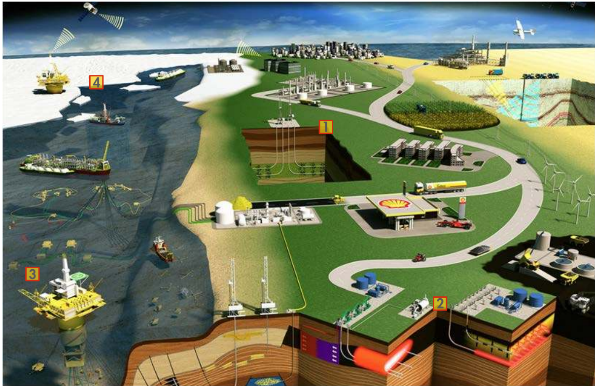
Figure 1.1: Integrated value chain of a state-of-the-art IOC and pictorial diagram of modern hydrocarbon recovery. ‘Easy oil’ is gone, advanced processes to extract more difficult resources have to be used and are the focus of the work presented in this thesis. The onshore field (1) uses fracturing techniques in long horizontal wells to extract gas or oil from shales. Steam is injected in onshore field (2) to lower the oil viscosity and consequently increase the recovery factor. New resources are increasingly found in challenging areas, such as deep sea environments (3) or in arctic conditions (4). All these more complex production conditions require monitoring to ensure efficient operation.
