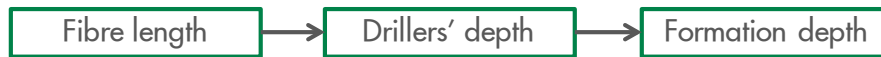
Figure 9.1: Typical calibration steps to achieve calibration from measured fibre length to position in the formation.
