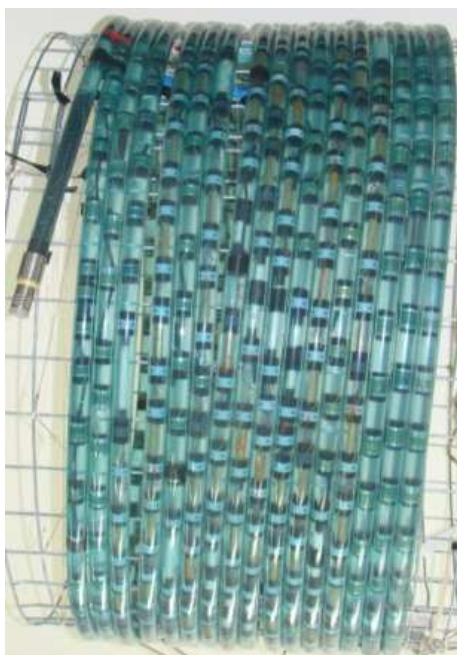
Figure 2. FOTA Array section wound on calibration drum
