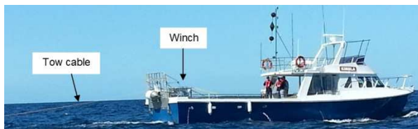
Figure 4. Support vessel towing the FO Array
