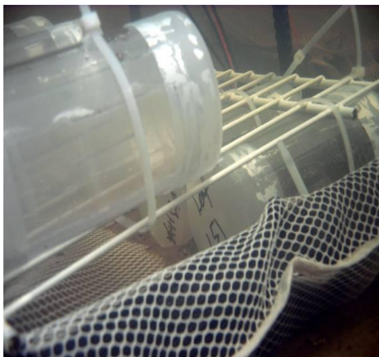
Figure 2. Underwater image showing the placement of the in situ toxicity chambers. One set of chambers was placed on the sediment/water interface and another set suspended in the water column.
