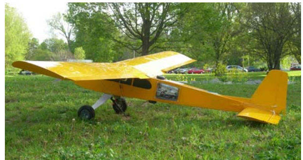
Figure 3. Electric powered Senior Telemaster with a 900MHz serial RF modem hosted in the middle section of the fuselage
