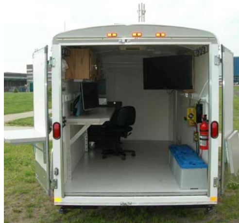
Figure 6. A mobile test support trailer to facilitate field experiments in UAV networking
