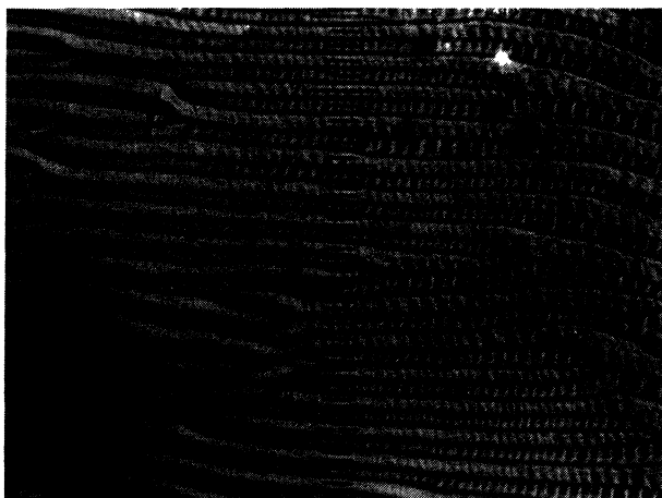
FIG. 4. — Pretransitional regime of distortion in a M24 planar sample. The stripes are parallel to \mathbf{n}_0 . The right part corresponds to the completely smectic region of the sample.
