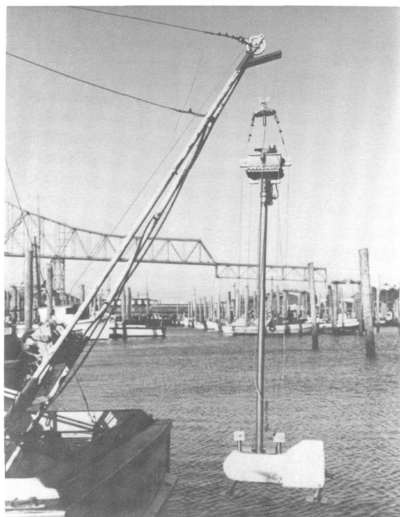
Figure 19.--Vibra-core sampler prepared for coring (core barrel approximately 5 feet long). From Prych and Hubbell, 1966, plate 1.
