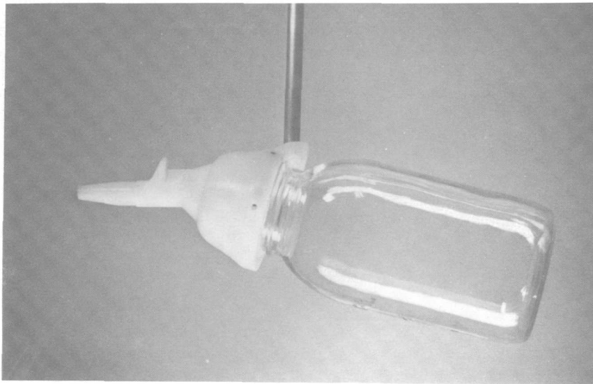
Figure 2.--US DH-81 suspended-sediment sampler.
