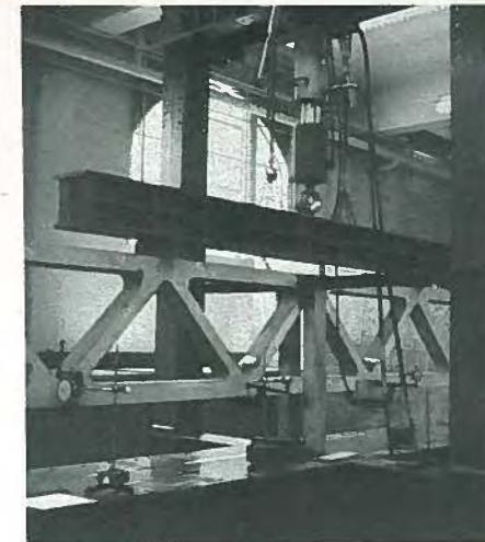
Fig. 25. Prototype truss undergoing testing in laboratory.
