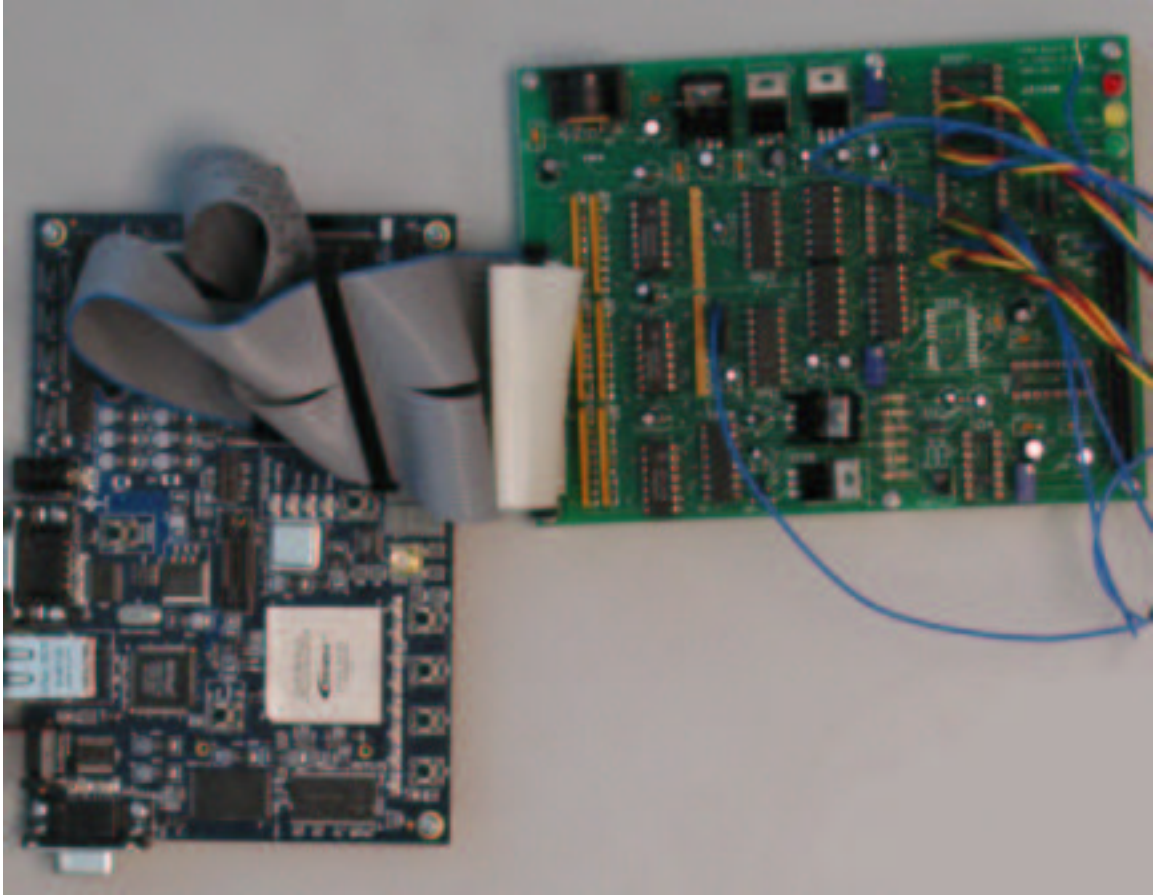
Figure 56. This is a picture of the mixed-signal prototyping platform. It is currently comprised of an off-the-shelf FPGA development board and a custom daughter card developed for the FPAA.
